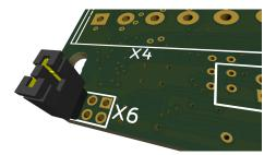
X6 Jumper Closed (Connected)
