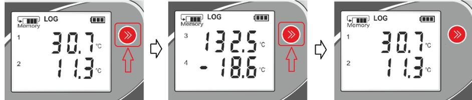
The lower push button serves to toggle between the currently measured values and the Min/Max values:
